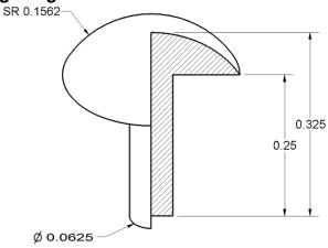
Note: Optional chamfer bottom edge .01 x 45 deg
