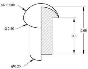
Note: Optional chamfer bottom edge .01 x 45 deg
