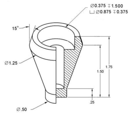
Note: Optional chamfer bottom edge .01 x 45 deg
